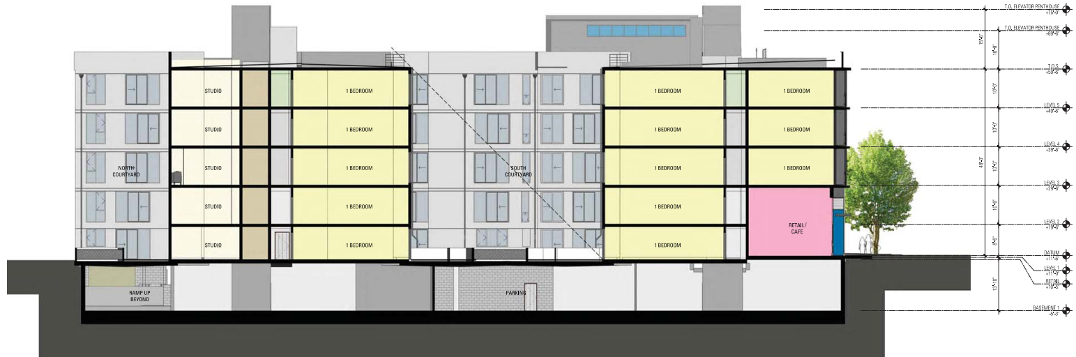
ⓑ NORTH/SOUTH SECTION THROUGH COURTYARDS
