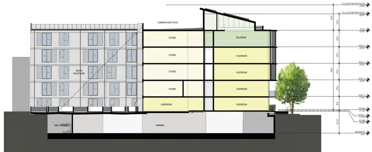
ⓐ EAST/WEST SECTION THROUGH SOLARIUM
